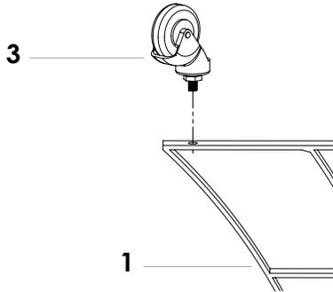
Secure caster wheels with large nut (B). To keep support brackets level, ensure the bolt on the wheel does not extend the large nut.
