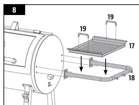
**IMPORTANT: Avoid using the side shelf handle to move or lift the grill. The weight of the unit will cause the side shelf handle to bend or break, which is not covered by warranty.**
